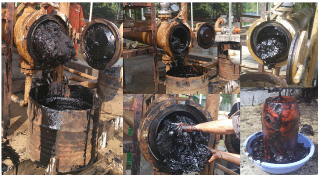
VKVC LLP: VKVC foam pigs to treat wax build up in crude oil pipelines.
