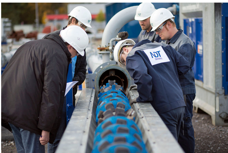
NDT Global: High resolution ultrasonic inspection tools identify the true state of corrosion in a pipeline.
