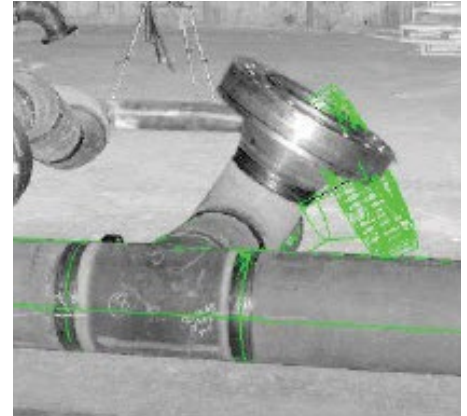
Fabricated spool doesn't match design
