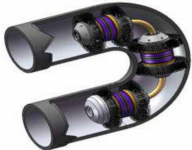
Figure 1. Intelligent Pig Navigating Piping
