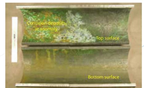
Figure 3. View of top and bottom interior surfaces of the tube
