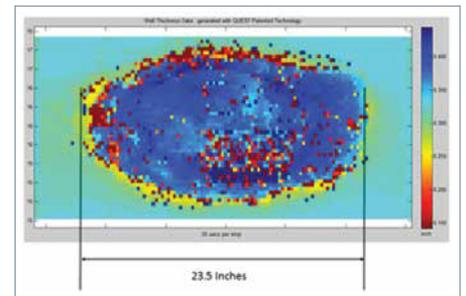
**Figure 5. Second inspection (one year later) results showing anomaly**
