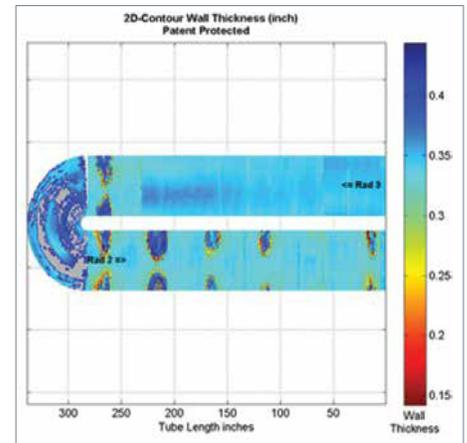
Figure 1. Anomalies as seen in two tubes joined by a return bend
