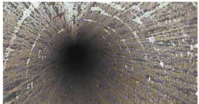
Figure 1. RDVI visual images show the extent of the damage within the convection section of the piping.
