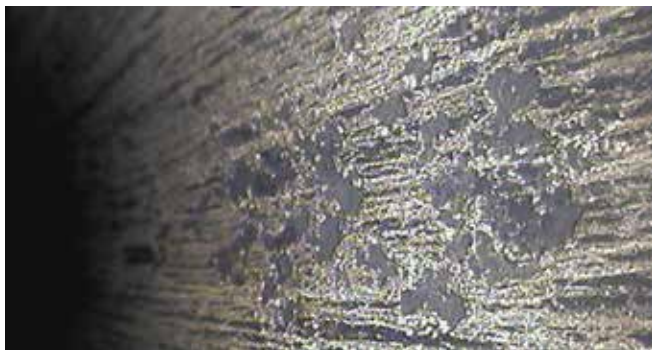
Figure 1. RDVI visual images show the extent of the damage within the convection section of the piping.
