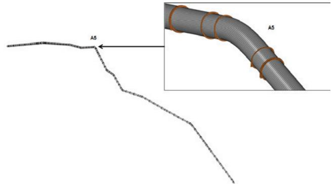
Figure 5. Example of structured finite element mesh used for all three penstocks.
