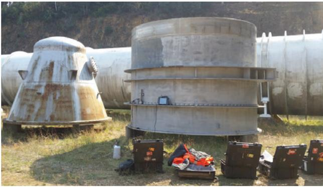
Figure 7: Removed section of penstock used for ToFD calibration.
