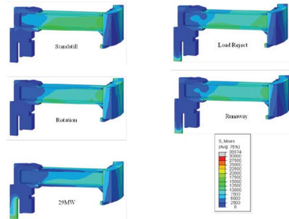
Figure 4. Finite element analysis (FEA) results that were used as the basis to determine the rotor spider's fitness-for-service.
