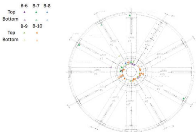
Figure 2. Example of rotor spider that was experiencing cracking in welds.
