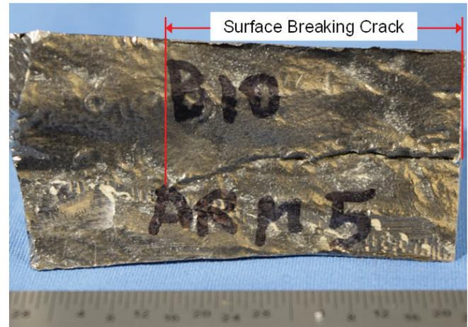
Figure 3. Crack located in the weld face metallurgical sample.
