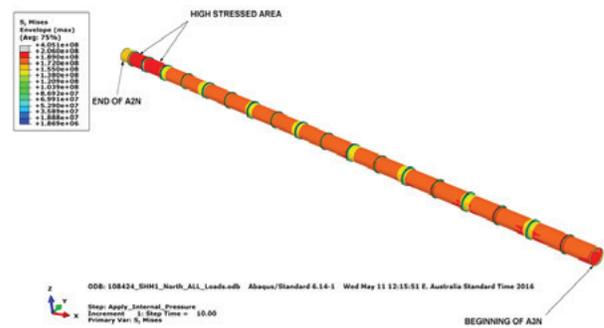
Figure 6: Example of stress results in penstock section A2N to A3N.
