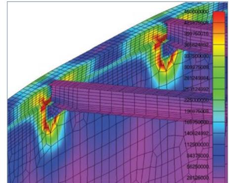
**Figure 4. Stress analysis of a fixed roof connection**
