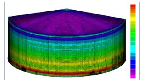
**Figure 2. Hoop stress due to hydrostatic pressure**
