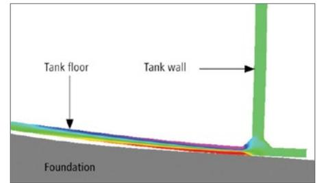
**Figure 3. Floor settlement stress results on an axisymmetric model**
