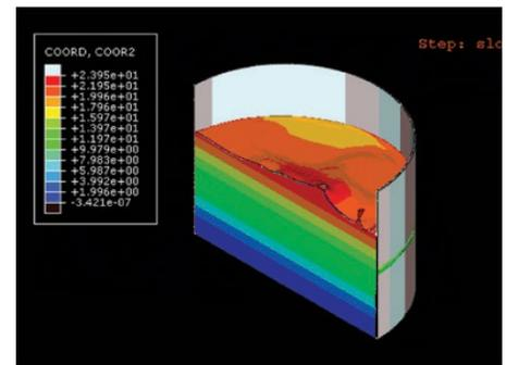
**Figure 1. Dynamic analysis of tank subject to earthquake loads**
