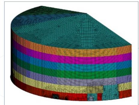
**Figure 5. 1/2 symmetric model of storage tank with repairs**
