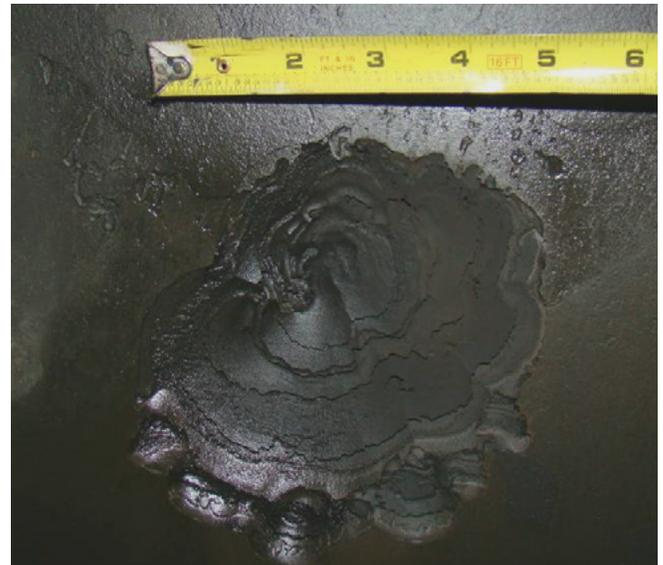
Figure 3 – CO<sub>2</sub> Corrosion, LTA
