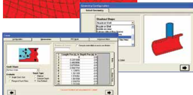
Choose from an extensive library of structural geometries and crack shapes. Advanced crack analysis allows the user to place a local 3D mesh anywhere in a global model.
