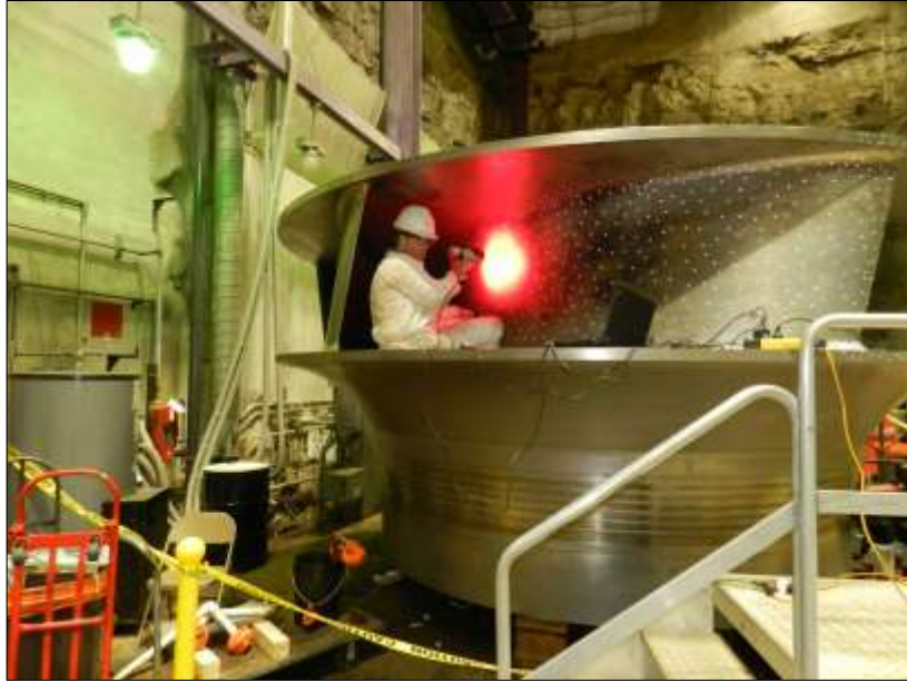
Figure 2: Quest Integrity engineer conducting a 3D laser scan of the high pressure side of the runner blade.
