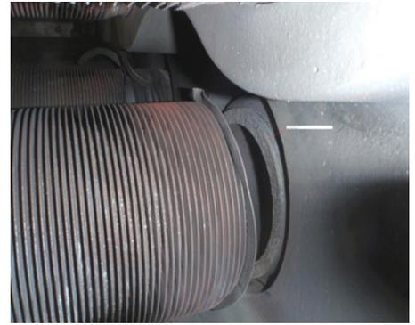
Figure 1. Tube failure at center support
