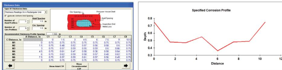
Figure 5. Example of LTA Data in Quest Integrity's Signal™ FFS engineering software.
