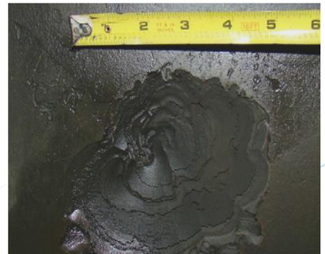
Figure 3. CO<sub>2</sub> corrosion, LTA
