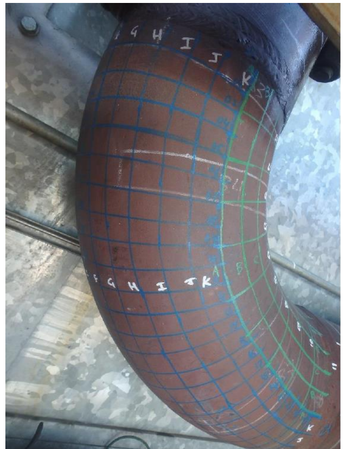
FIGURE 3: ULTRASONIC THICKNESS READING ON GRID ACROSS ELBOW. READINGS USED IN FFS ASSESSMENT.
