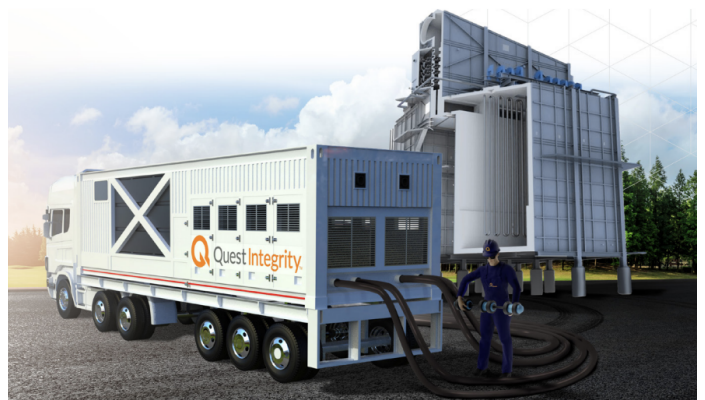
Figure 3. Typical Fired Heater Set Up for Advanced Cleaning and FTIS Inspection
